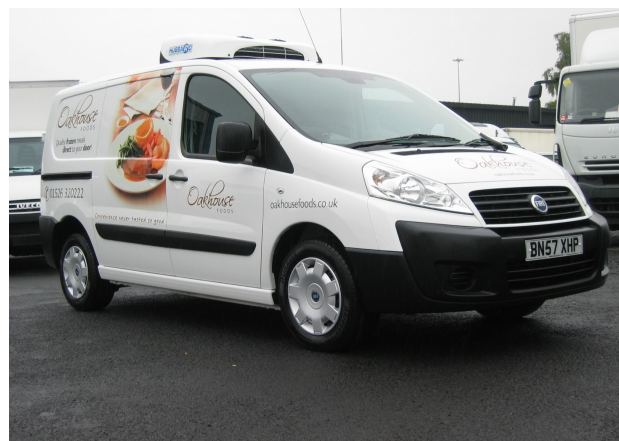
Fiat Scudo refrigerated panel van; specified and converted by Vanfridge Ltd, for Oakhouse Foods franchise in Metheringham, Lincolnshire, showing Hubbard 390 Alpha L fridge units.
