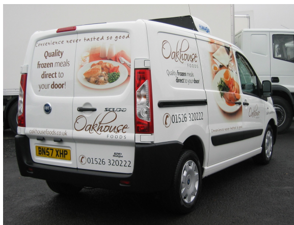
Fiat Scudo refrigerated panel van; specified and converted by Vanfridge Ltd, for Oakhouse Foods franchise in Metheringham, Lincolnshire, showing Hubbard 390 Alpha L fridge units.
